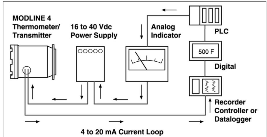
Modline 4 two-wire transmitter diagram
