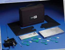
The temperature profile that the module is subjected to during the lamination process is critical to the correct curing of the ethylene vinyl acetate (EVA) and as such, has a direct effect on module lifetime. Datapaq SolarPaq temperature profiling systems enable the process to be monitored without disrupting normal production. The logger and its associated thermocouples are placed into the laminator, along with the module to be monitored.
