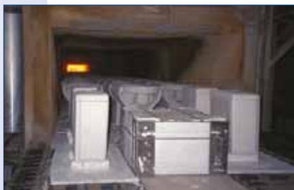
Kiln Tracker system in roller hearth sanitaryware kiln
