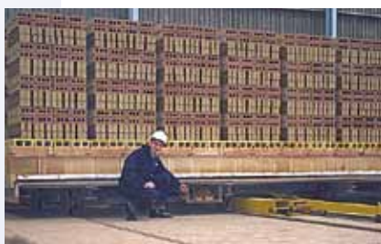
Kiln Tracker system beneath kiln car monitoring clay blocks
