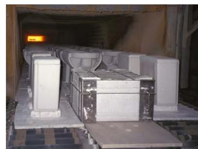
Kiln Tracker system in roller hearth sanitaryware kiln
