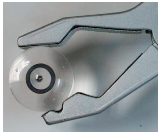
Figure 2: An example of an injection-molding product is the laser pick-up for compact disc players. It consists of an aspherical optical lens with a diameter of 4 mm whose conformity to the mold is within 0.1 thousandth of a millimeter. When this component leaves the mold it is ready for final assembly.
