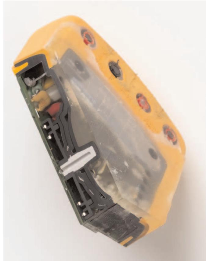
This DMM has been filled with resin and then sliced open, allowing Fluke mechanical engineers to see how the contact points line up.
