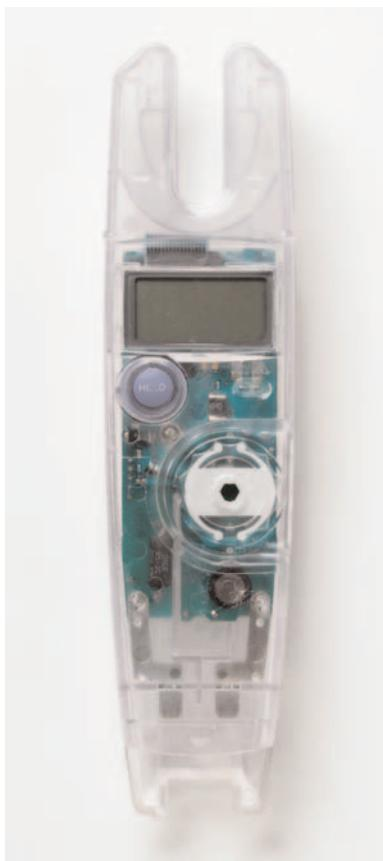
Fluke mechanical engineers create these see-through prototypes so they can watch the effects of twisting, prying, and shaking on the tool's innards.
