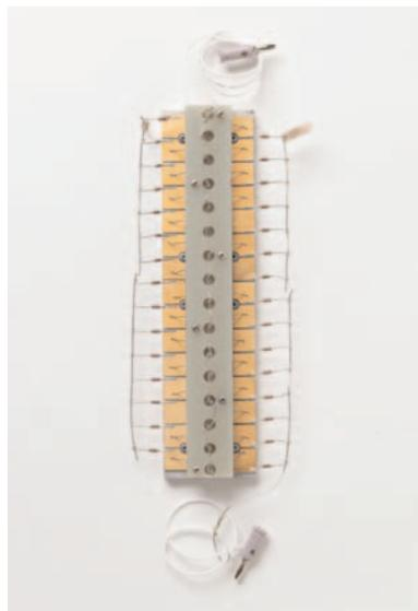
This battery contact test board tests different material combinations, including wire thickness, contact pad metal composition, and lubrication requirements. The goal: the strongest electrical connection to the battery.
