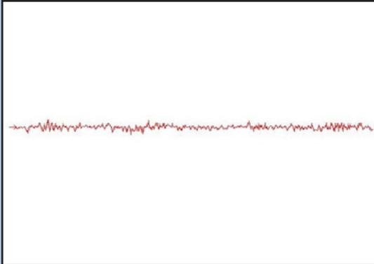
**Early bearing damage time domain signal**
