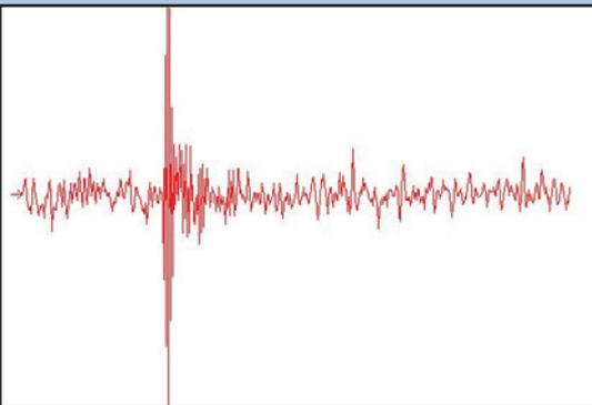
**Heavy bearing damage time domain signal**
