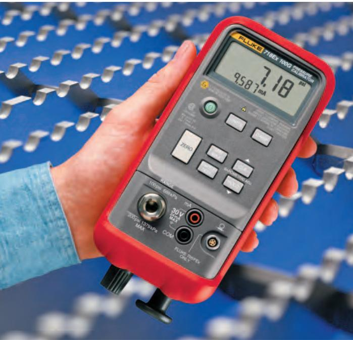
Pressure calibration can be a difficult challenge in the best of environments. Doing so in an area that has the potential for explosion takes the degree of difficulty to another level—one where the technician needs proper training and equipment. This article will demonstrate the practical application of pressure calibrators designed to perform calibrations in potentially explosive environments.
