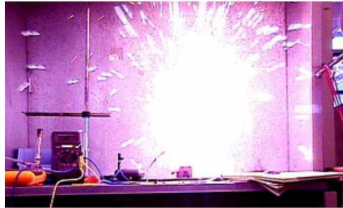
the high temperatures (up to 10,000 °F) generated by the energy will melt the sand and turn it to glass. The glass coats the element and smoothes the fireball by cutting off the available oxygen, keeping you and the tester safe from harm.
