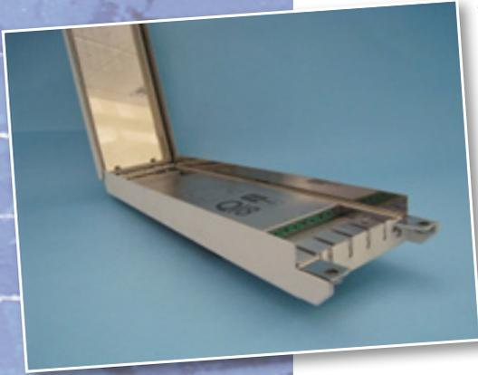
The Datapaq® SolarPaq system has been designed specifically to monitor the temperature of the glass substrate as it passes through the vacuum coating process. The profiling system passes through the multichamber process measuring the temperature profile from up to 4 positions on the glass; even with the plasma activated. This feature combined with the unique reflective plate thermal barrier enables the system to be used without disrupting normal production flow.
