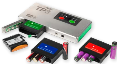
User replaceable battery options (NiMH, alkaline, Hi-temp)
