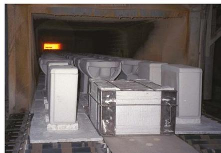
Kiln Tracker system in roller hearth sanitaryware kiln
